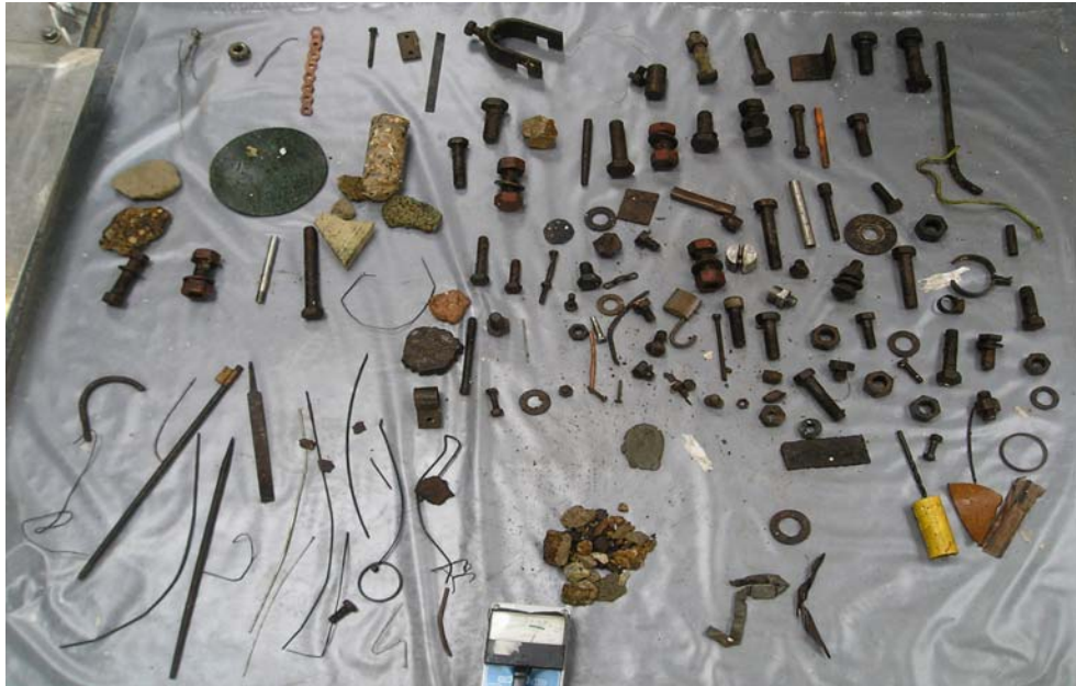
Figure 2: Examples of Mixed Debris Items Recovered from EAST Tanks
