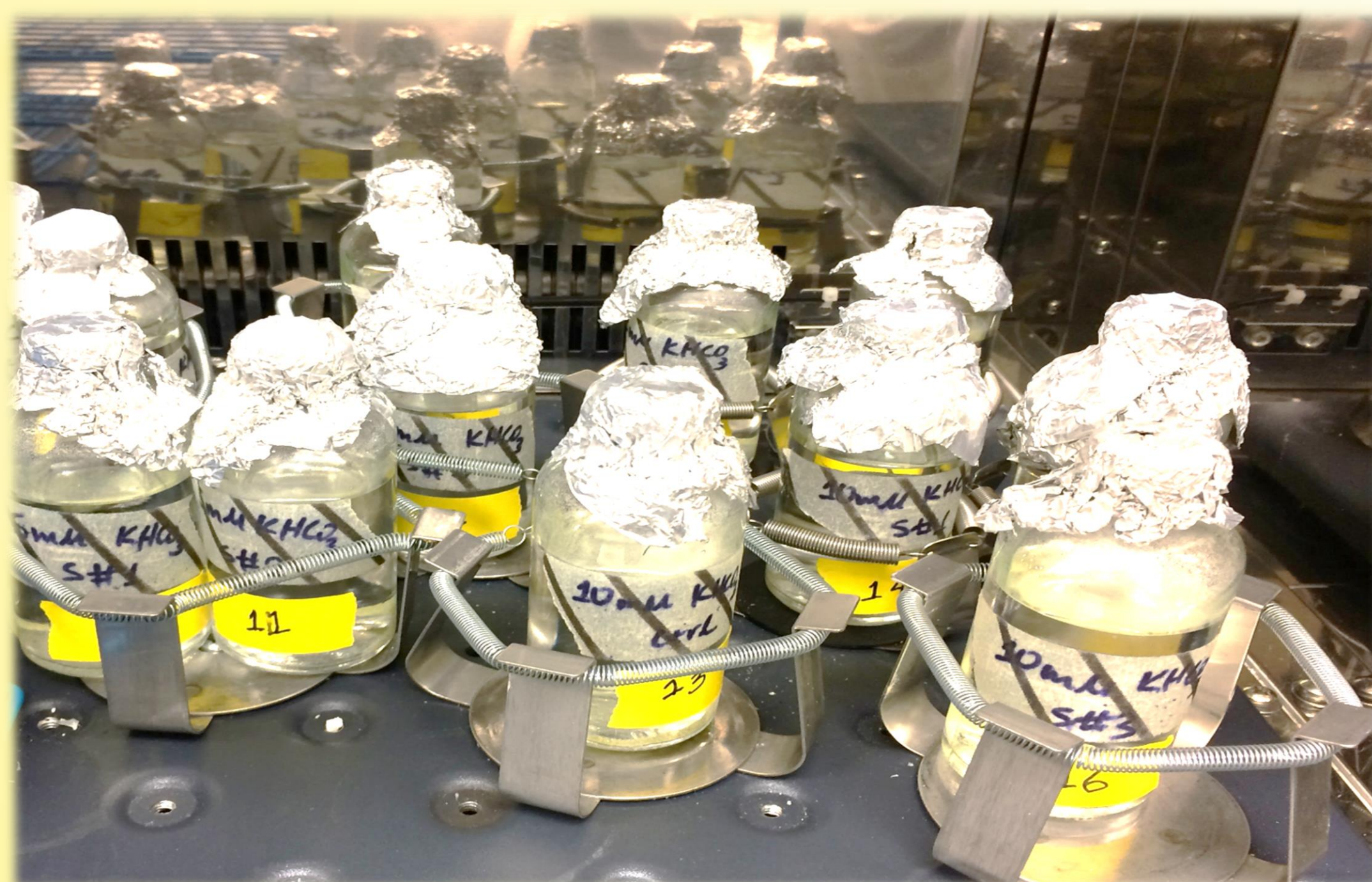
Figure 1. Experimental bottles for Ca-autunite dissolution.
