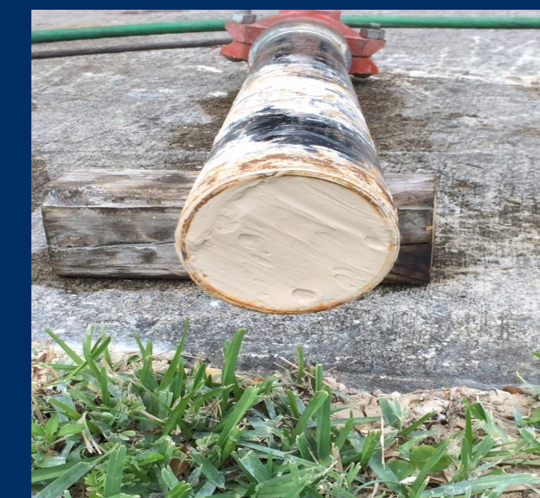
Figure 4: Plug blowout test.
