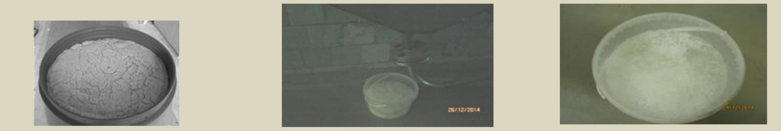
The appearance of the sample after solidifying the evaporator cube residue. The total \alpha -activity was 2.5 \cdot 10^6 Bq/kg; the total \beta -activity was 7.3 \cdot 10^7 Bq/kg.
