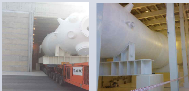
Figure 1. Storage of old Steam Generator
