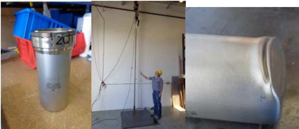
Figure 17. New 2 Qt. 3.7 meter (12 ft.) drop test and result.
