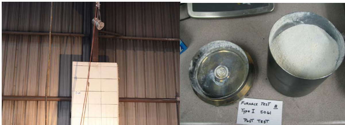
Figure 14. Drop Test: Type I Lid Impact Pre Test.
