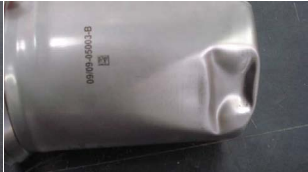
Figure 10. Side Drop Damage
