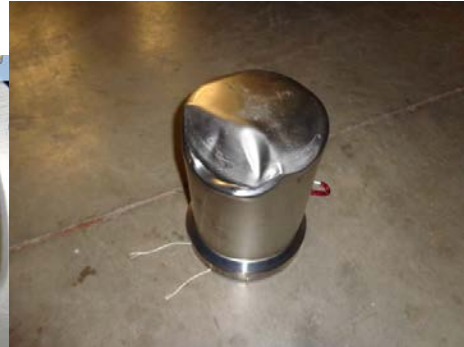
Figure 20-22. Results of the stacking, penetration and 9.2 m (30 ft) drop tests
