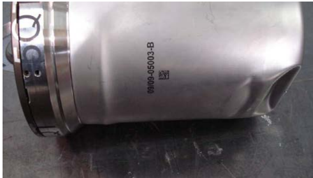
Figure 9. Slap Down Damage
