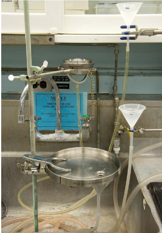
Fig. 15. Experimental setup for water Pen. Fig. 16. Water is seen on filter of SAVY after 2 hr. exposure to 15.3 cm (six in) of water column
