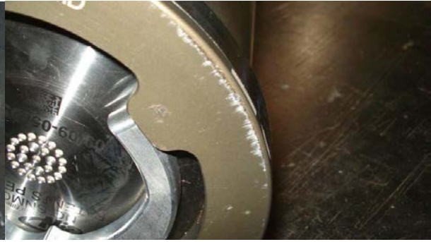
Figure 8. Top Flat Down Damage
