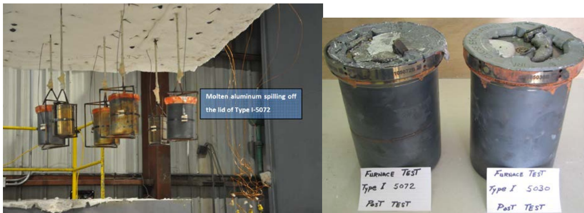
Figure 12. Furnace Test 1: Type 1 Containers Post Test.
