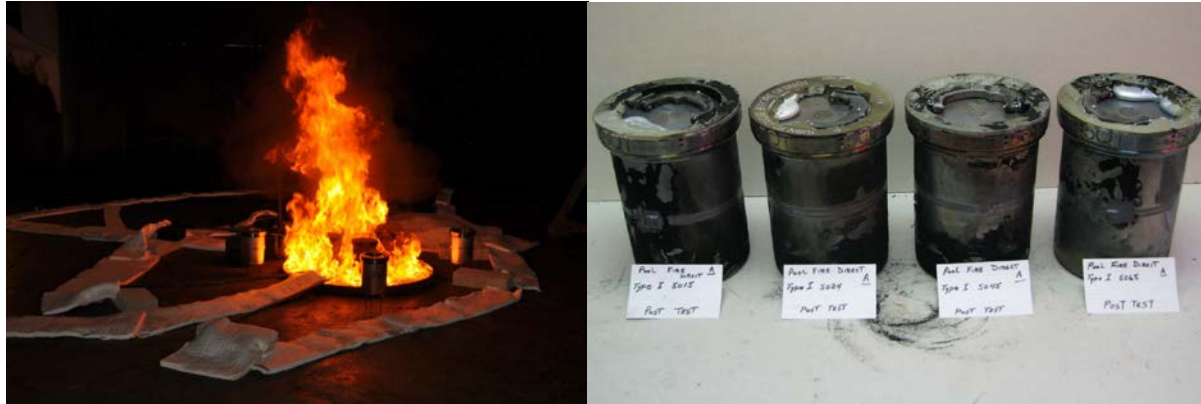
Figure 13. Open Flame Test 1: Full Ignition of Kerosene and Post Test Direct Exposure Containers.
