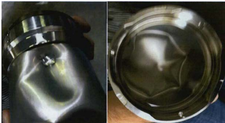
Figure 18. Damage caused by penetration bar test.
