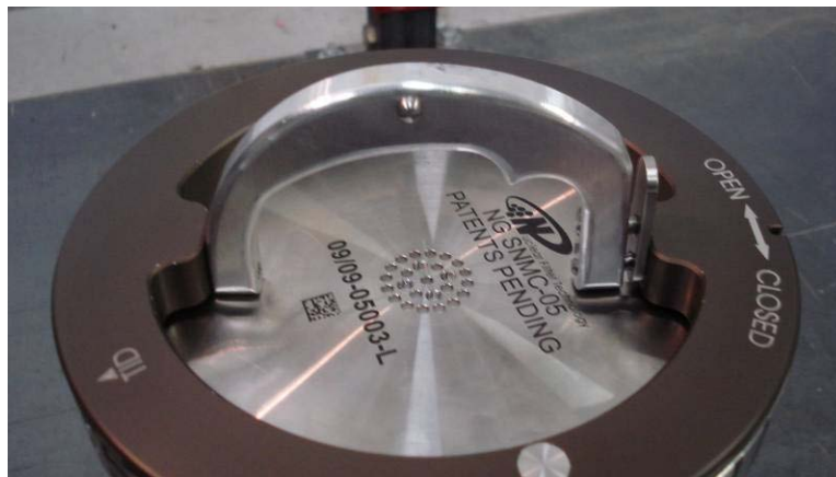
Figure 11. Top Down on Handle Damage
