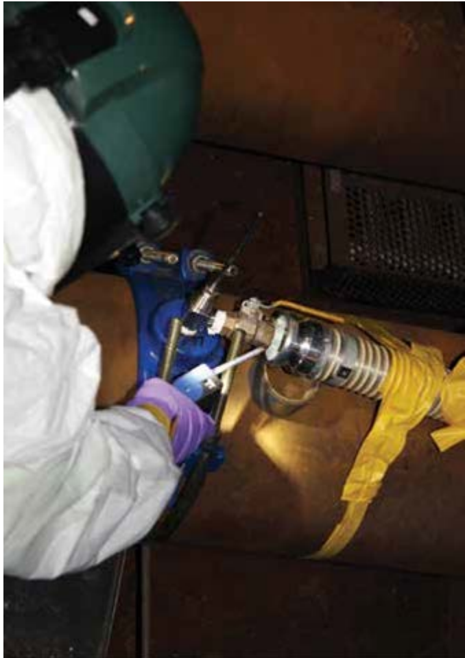
Fig. 4. A technician samples gases vented from a process gas system to verify the absence of hydrogen fluoride.
