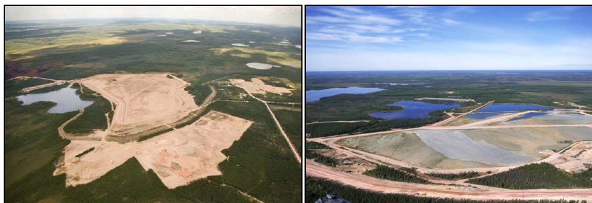
Fig. 9 Conventional Mill Tailings Impoundment During Mill Operations (Left) and Following Decommissioning (Right)
