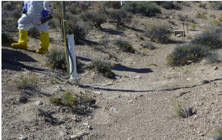
Figure 4. In Plutonium Valley, the Isco sampler and ultrasonic depth sensor are installed in the channel emanating from the southernmost test bed (top left). A close-up of the Isco sampler, which collects suspended-load samples during flow events, is shown (top right). A bedload sampler is located downstream of the ultrasonic depth sensor (top right corner of bottom left photo), with a close-up of the bedload sampler shown (bottom right).
