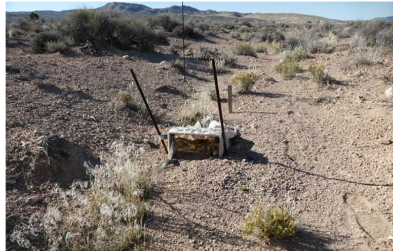
Figure 4. In Plutonium Valley, the Isco sampler and ultrasonic depth sensor are installed in the channel emanating from the southernmost test bed (top left). A close-up of the Isco sampler, which collects suspended-load samples during flow events, is shown (top right). A bedload sampler is located downstream of the ultrasonic depth sensor (top right corner of bottom left photo), with a close-up of the bedload sampler shown (bottom right).
