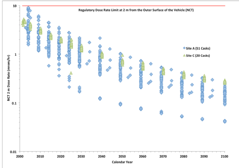
Fig. 5. Maximum NCT Dose Rates at 2 m from Cask Surface as a Function of Year for Sites A and C.
