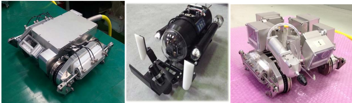
Fig. 6 – Picture of 3 IHI ROVs used in Inspection (Left-Right: Vent Tube, Down Leg, Suppression Chamber)
