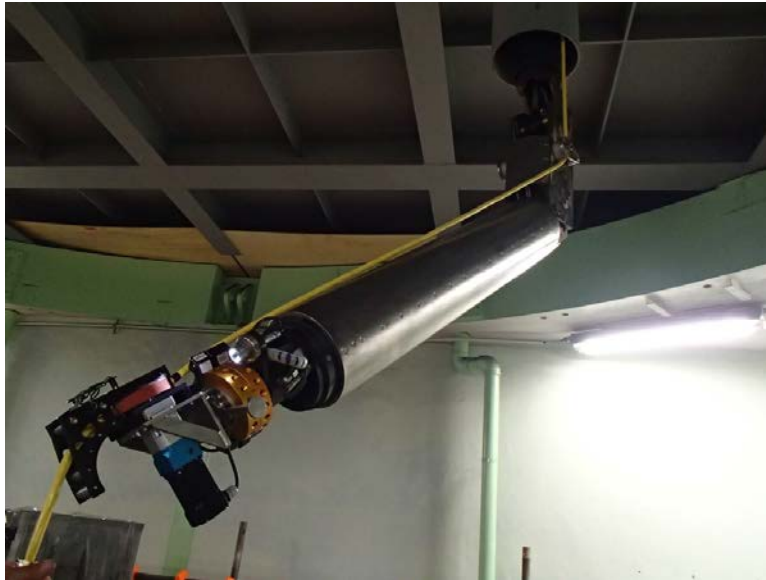
Fig. 7 – Picture of FIM and ROV Deployment Tool during Testing at IHI Mockup
