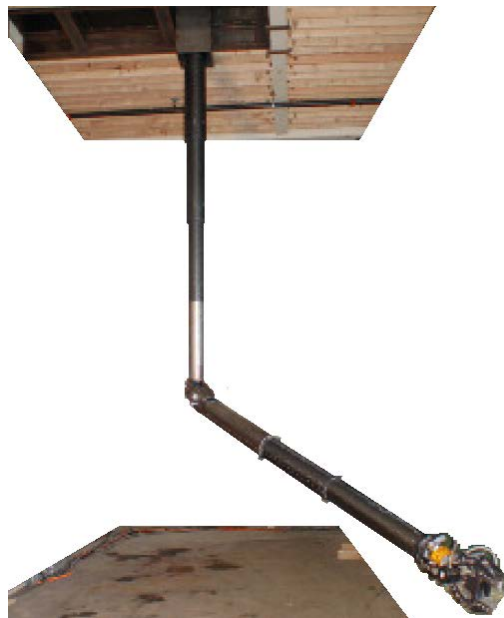
Fig. 5 – FIM Deployed in Colorado Mockup Demonstrating Long Reach Capabilities
