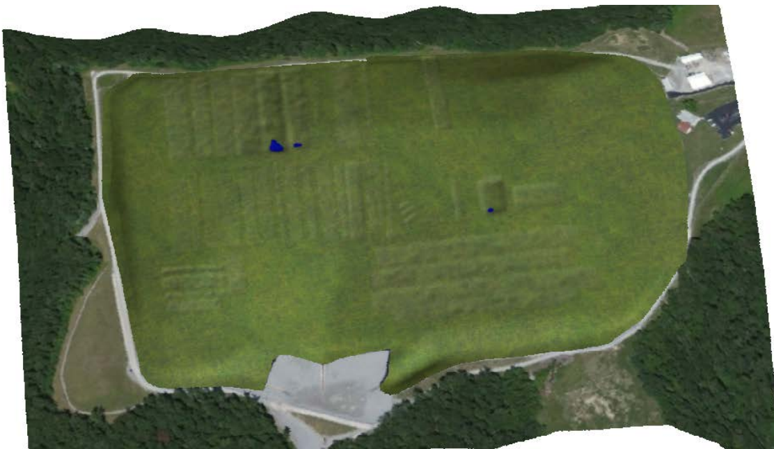
Figure 5. Example Realization of Differential Settlement Model of Final Cover System
