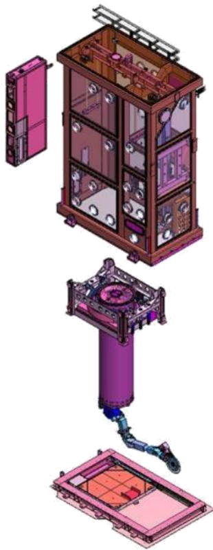
Figure3. Remotely-Operated Handling and Cutting Unit - 3D exploded view
