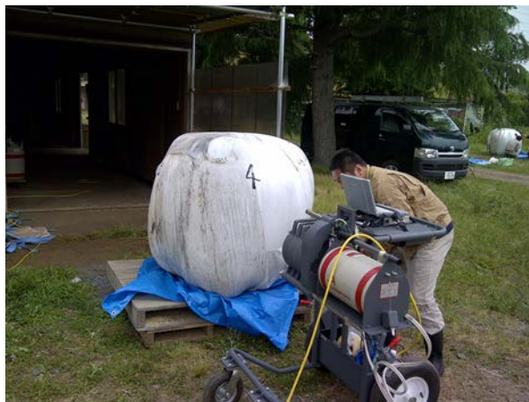
Fig. 5. The ISOCS in-situ Ge measurement
