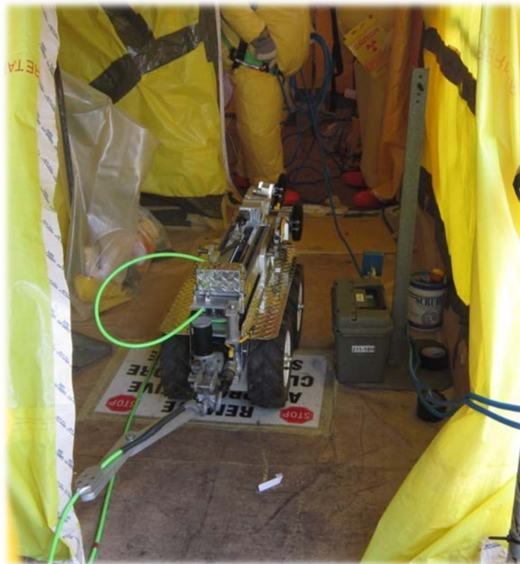
Fig. 15. Crawler Entering Hoist for Deployment
