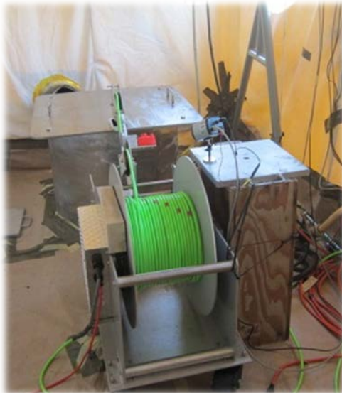
Fig. 11. Automated Tether Control Mechanism
