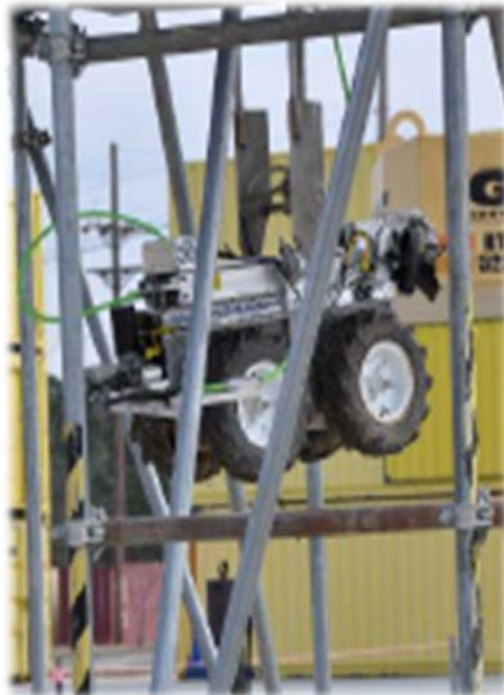
Fig. 13. Transition to Horizontal Rigging
