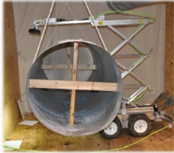
Fig. 7. Camera on boom mock-up
