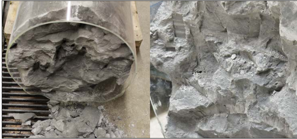
Fig. 13. Front face of the second backfill cylinder with the supercontainer models. Fragments of the backfill were chiseled out by hand and with a small electric concrete breaker.
