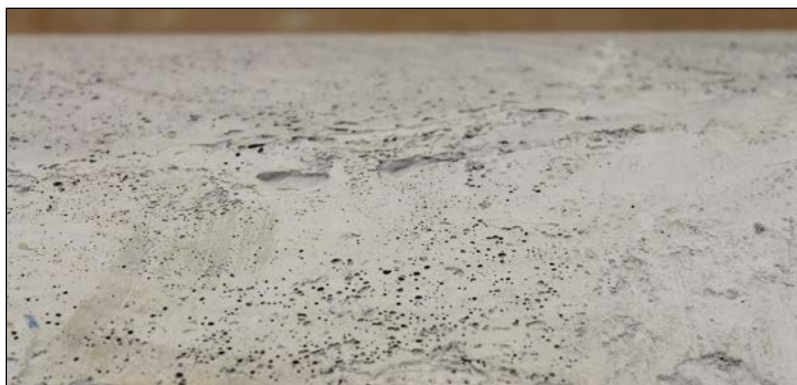
Fig. 11. Drill cores (diameter 10 cm) of the backfill tests illustrate the homogeneity of the backfill material. According to visual inspection, density and porosity measurements the upper parts of the cylinders have a slightly increased air pore content.
