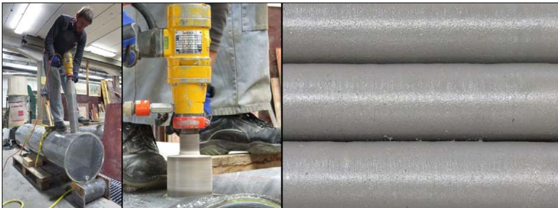
Fig. 11. Drill cores (diameter 10 cm) of the backfill tests illustrate the homogeneity of the backfill material. According to visual inspection, density and porosity measurements the upper parts of the cylinders have a slightly increased air pore content.
