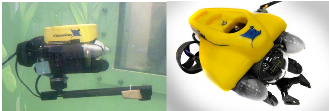
VideoRay Pro4 with boom camera in use in test tank Pro4 with gripper
