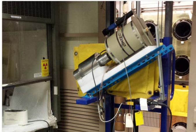
Fig. 2a – Liquid nitrogen cooled HPGe coaxial safeguards detector with wide FOV collimator
