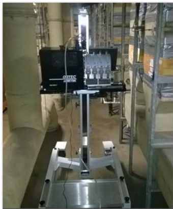
Fig. 2b – IDM-200-V Stirling cooled HPGe detector mounted on the ANTCart®
