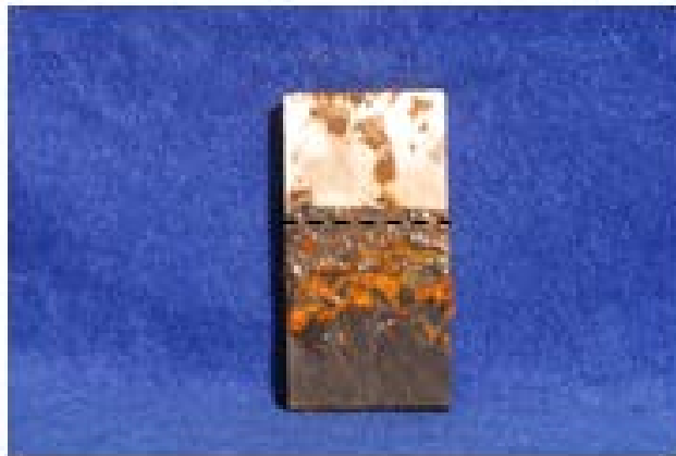
Fig. 9. Steel Specimen after Two Months 50% Submerged in Leak Detection Pit Water.
