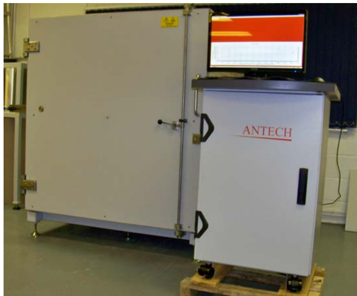
Fig. 1. Model CHF550-20800 Heat-flow Drum Calorimeter.
