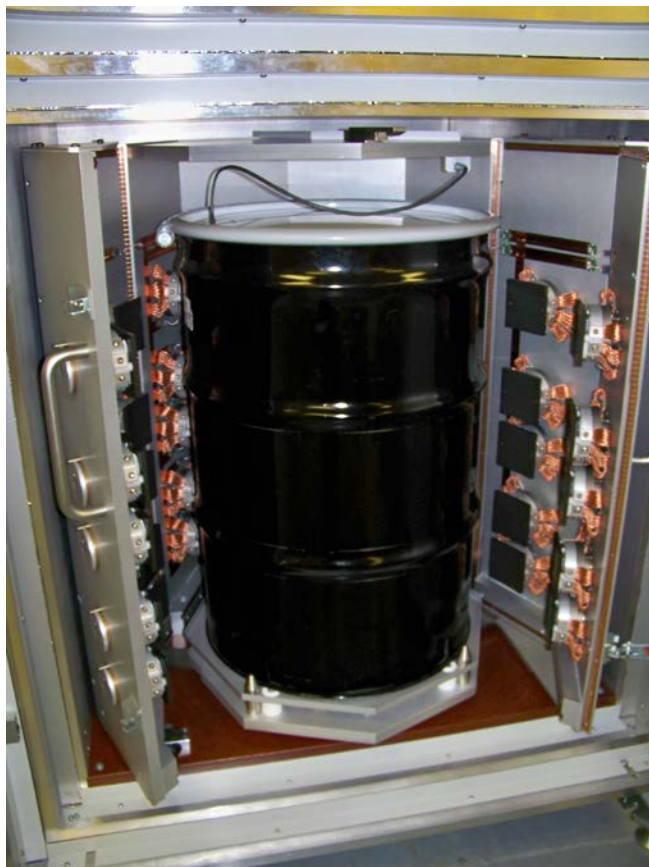
Fig. 3. Drum calorimeter with drum inserted into the octagonal heat sink chamber assembly in the open or loading/unloading position.
