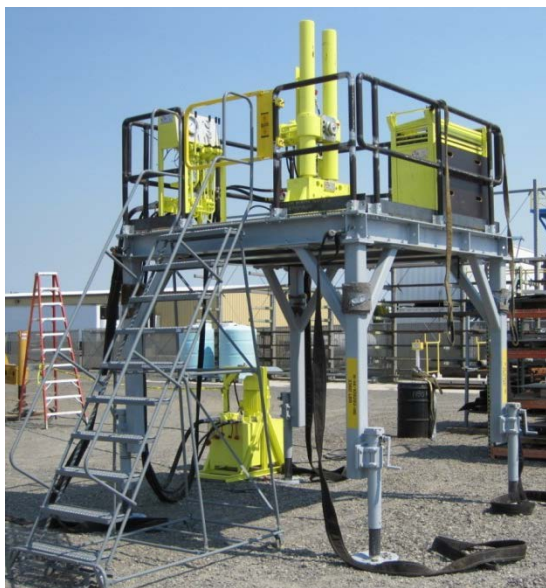
Fig. 1. Cone Penetrometer Test Platform
