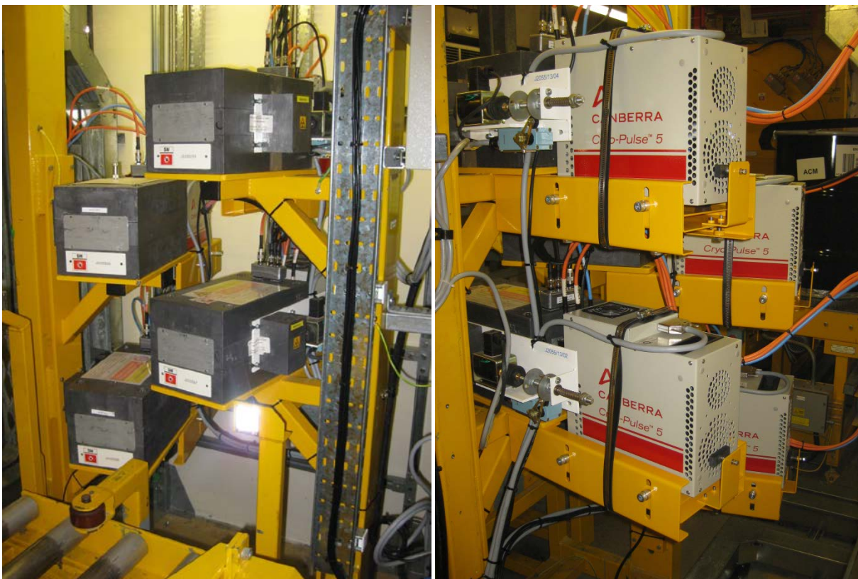
Fig. 1. The four detector Drum HRGS used for the measurements. The left image shows the collimators pointing toward the drum cavity. The light gray rectangle above the white label is the Cd filter. The right image shows the electrical cooler.
