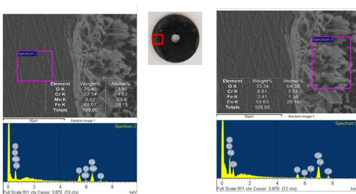
Fig. 5. SEM/EDS result of synthesis of CRUD on metallic coupon
