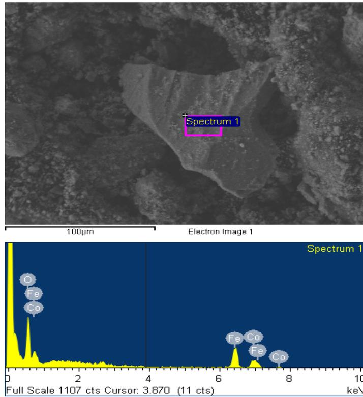
Fig. 3. SEM/EDS result of  $\text{CoFe}_2\text{O}_4$
