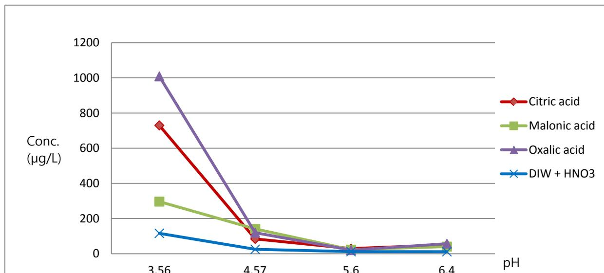
Fig. 6. The concentration of Co with different chemical reagent and pH in dissolution test
