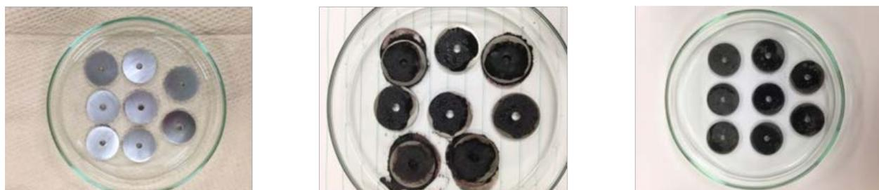
Fig. 4. Synthesis of CRUD on metallic coupon
