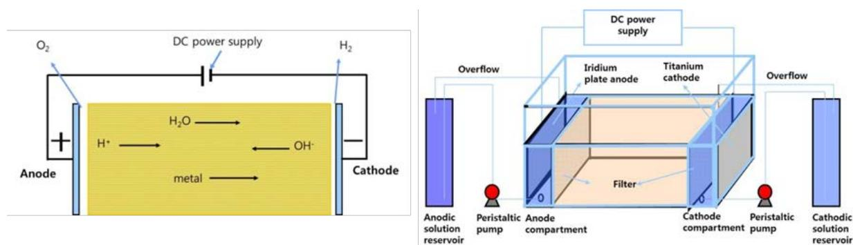
Fig. 1. Schematic diagrams of the experimental apparatus (EK process)
