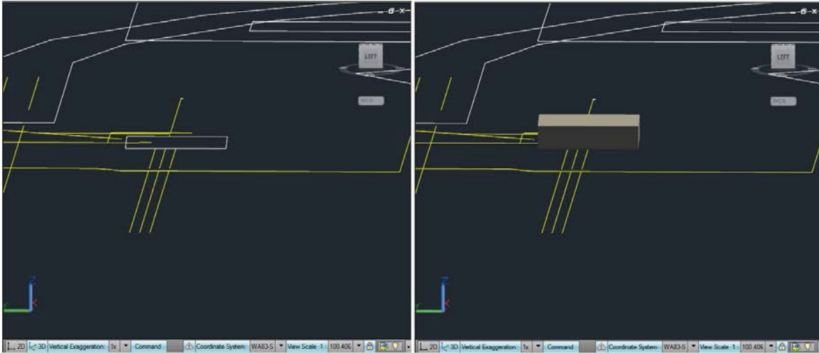
Fig.1.-Extruding a Rectangular Waste Site Shape File.
