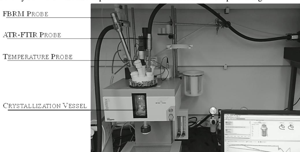
Fig. 1. Optimax™ workstation equipped with focused-beam reflectance measurement (FBRM) and attenuated total-reflectance Fourier transform infrared (ATR-FTIR) online measurement technology.
