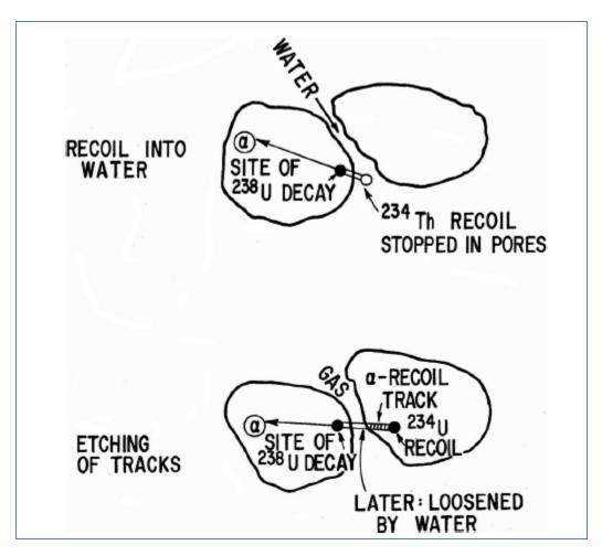
Figure 3 – Alpha Recoil Process
