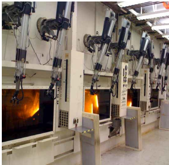
FIGURE 2. AGHCF work stations with ZnBr-filled windows for viewing and remote operations in the hot cell.
