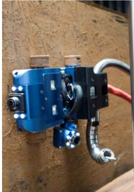
Fig. 12 – Delivery platform – SWATS Service equipment – Camera & retrieval tool
