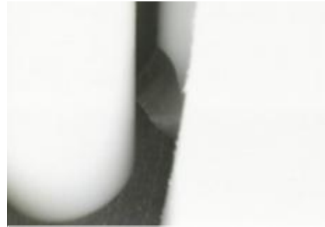
Fig. 9 – BICS image, machining remnant in a gap of 0.116" (2.95mm) gap
