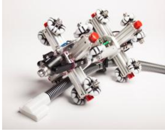
Fig. 13 – ROV – Pipe walker FOSAR system
