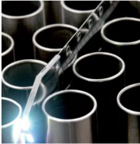
Fig. 8 – Brooks In-Bundle Camera System (BICS) – width 0.100" (2.54mm)
