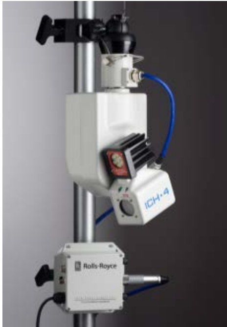
Fig. 1 – ICH-4 Camera & Local Power Supply utilizing quick connect pole mount
