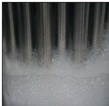
Fig .13. Decontamination foams
