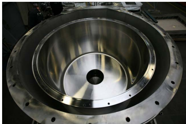
FIGURE 3. Stainless steel mixing pan with cone-shaped bottom and opened discharge gate - encircled by the low pressure casing
