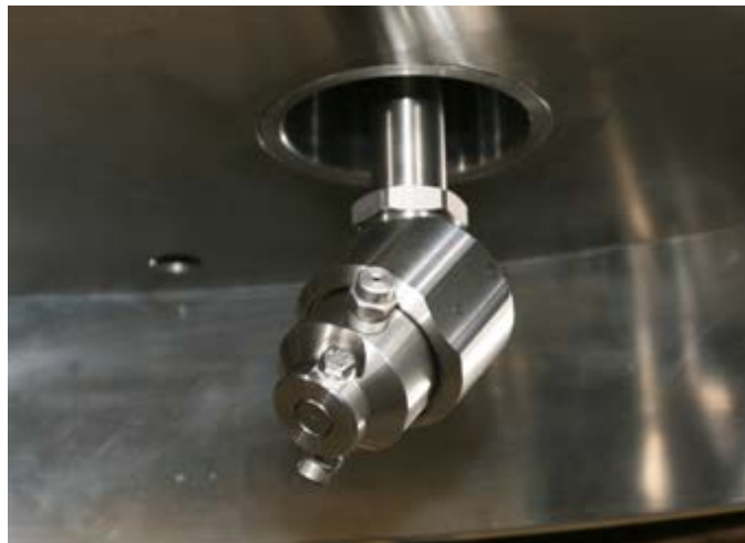
FIGURE 5. Rotational cleaning nozzle installed in the upper cover of the mixer
