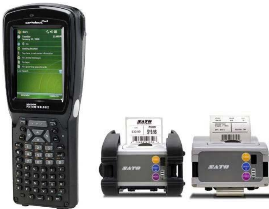
Fig. 5. Mobile computer and field printer support field operations like waste identification.
