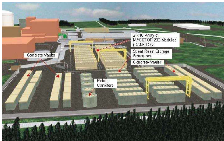
Figure 10 – Illustration of CANDU® 6 Waste Management Facility with MACSTOR® Technology planned for Gentilly-2 (Canada)
