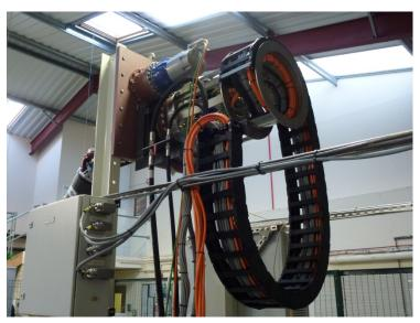
Figure 3 - Out-Cell Shoulder Drive & Valve Pack
