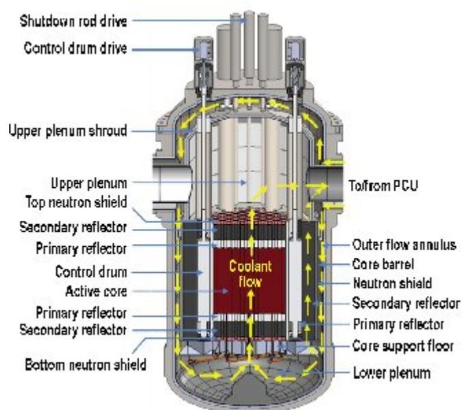
Fig. 2. Cutaway of EM<sup>2</sup> reactor system.
