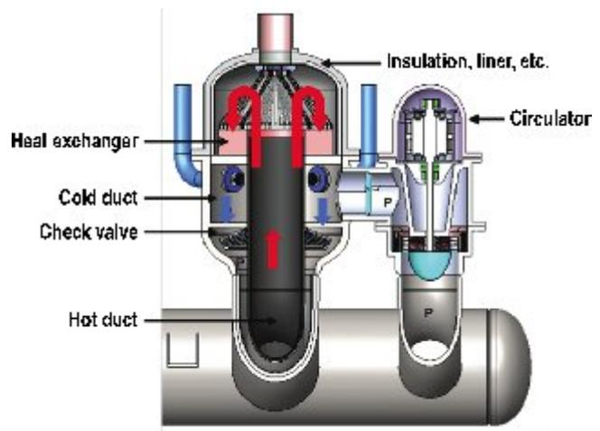
Fig. 5. DRACS heat exchanger cutaway.
