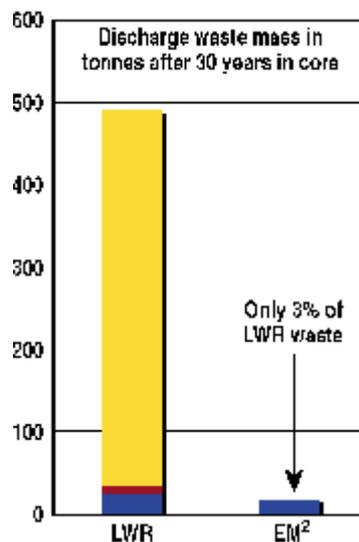
Fig. 18. Comparison of the net waste in tons after 30 years of operation for 1.2 GWe advanced LWR and EM<sup>2</sup> plants.
