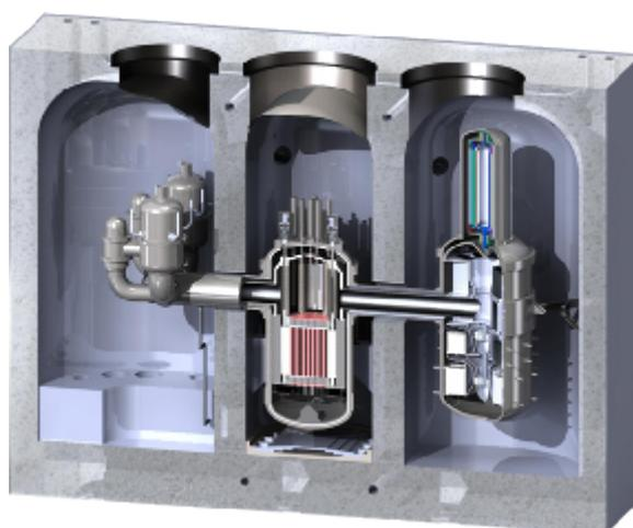
Fig. 1. 250 MWe EM<sup>2</sup> power module in a below-grade sealed containment.
