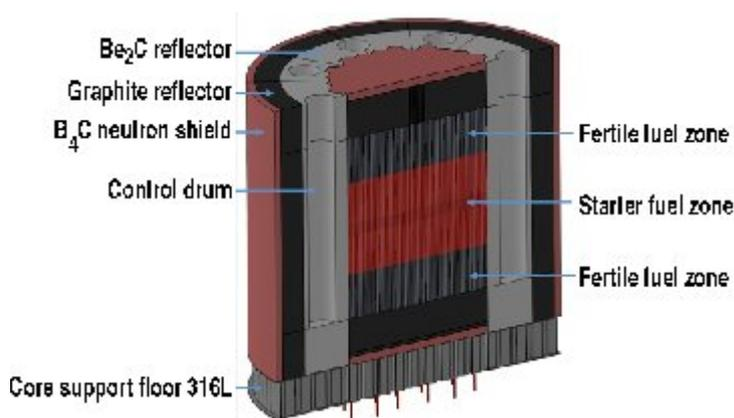
Fig. 3. EM<sup>2</sup> core arrangement composed of starter and fertile sections. (The shapes of the fissile and fertile sections are only schematically illustrated.)
