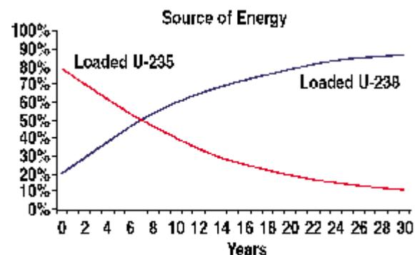
Fig. 7. Fractional contribution of loaded material to core power over time.
