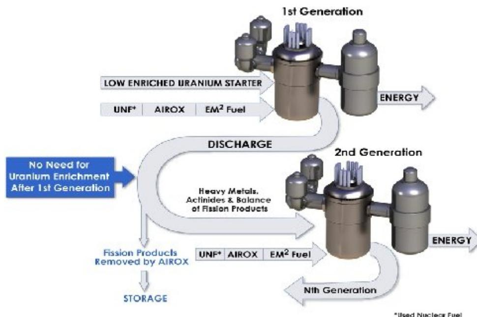
Fig. 10. Illustration of EM<sup>2</sup> closed fuel cycle without conventional reprocessing.
