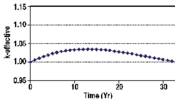
Fig. 6. Neutronics calculation showing a 30+ year core life and the tight control range of k-effective for EM<sup>2</sup> core fueled with LEU and DU.
