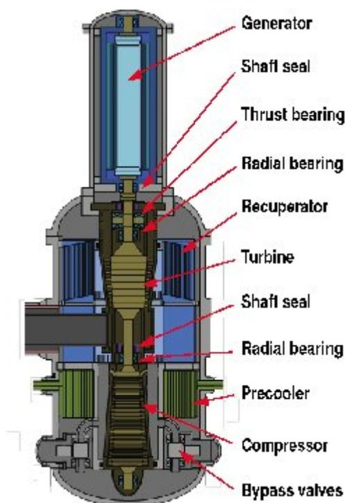
Fig. 4. PCU and generator cutaway.
