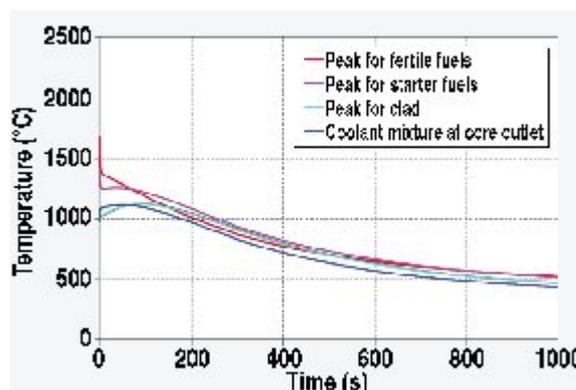
Fig. 9. Pressurized natural convection cooldown on one DRACS loop.
