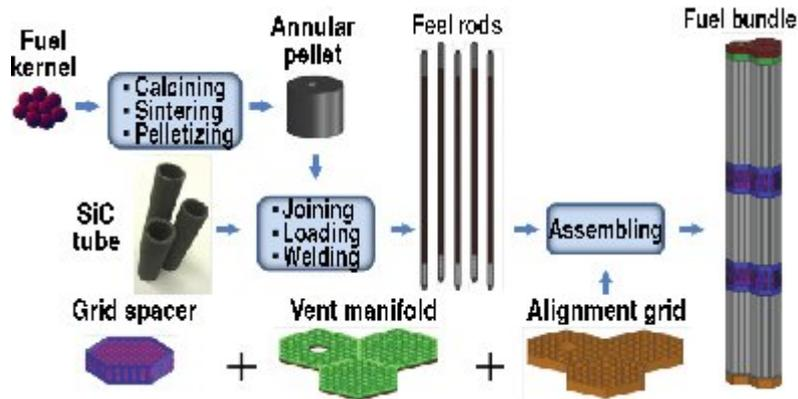
Fig. 11. EM<sup>2</sup> fuel manufacturing process.
