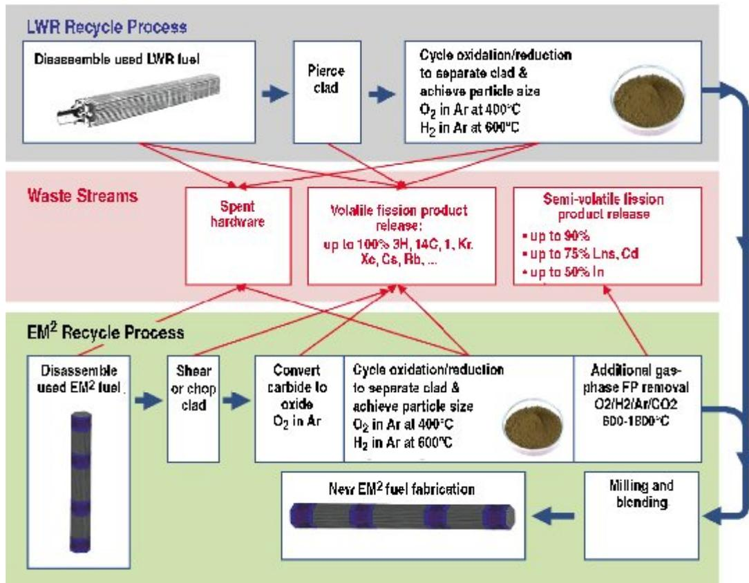
Fig. 12. Adaptation of voloxidation process to proliferation resistant re-fabrication of LWR and EM<sup>2</sup> fuel.
