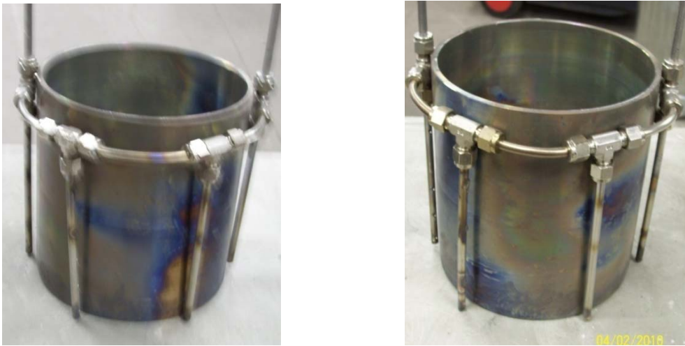
Figure 11. Two views, front side/back side, of the thick wall stainless steel container at the completion of the glass melting experiment. Non uniform tarnishing is evident, but oxidation is minimal or non-existent.
