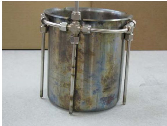
Figure 4. Appearance of the outside surface of the stainless steel can after two induction melting experiments. The four short cooling tubes provided air cooling during the melting experiments. The can is in good shape and shows what is considered only minor oxidation. In the second scoping experiment where the borosilicate glass was melted, the can reached a maximum temperature of \sim 700\text{ }^{\circ}\text{C} and the maximum temperature of the graphite crucible/susceptor was 1075^{\circ}\text{C} .
