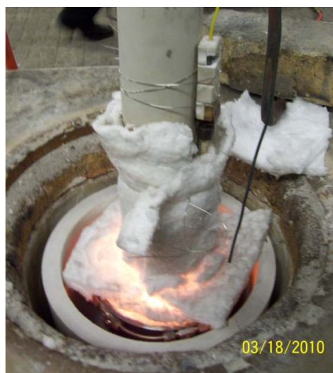
Figure 7. Induction melting of borosilicate glass, BS AN-104, 2.5 hrs after start. Temperature of graphite crucible was 1075 °C. The melt was fluid with a consistency of honey.
