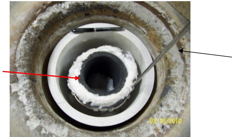
Figure 5: Photo showing graphite crucible/stainless can assembly inside ceramic safety crucible. White fiber insulation (red arrow) is placed between graphite and stainless can to insulate the stainless can from the hot graphite crucible. Black arrow points to air cooling tube and the fountain pen placed on the safety crucible is scale marker.
