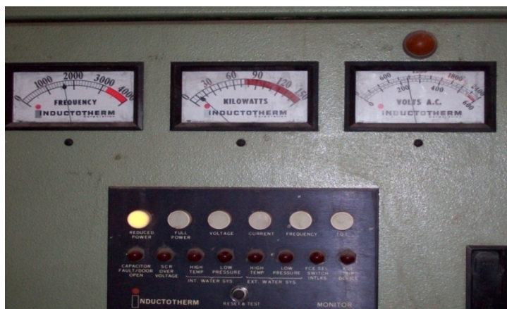
Figure 2. General view of the control panel of the induction power supply used for the glass melting experiments.
