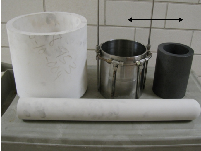
Figure 9. Ceramic safety crucible (left), thick wall (0.182 inches) stainless steel container (middle), equipped with air cooling device, graphite crucible (right) and ceramic melter tube (in front). In the induction melting experiment the stainless container, graphite crucible, and ceramic melter tube were placed inside the large ceramic safety crucible.
