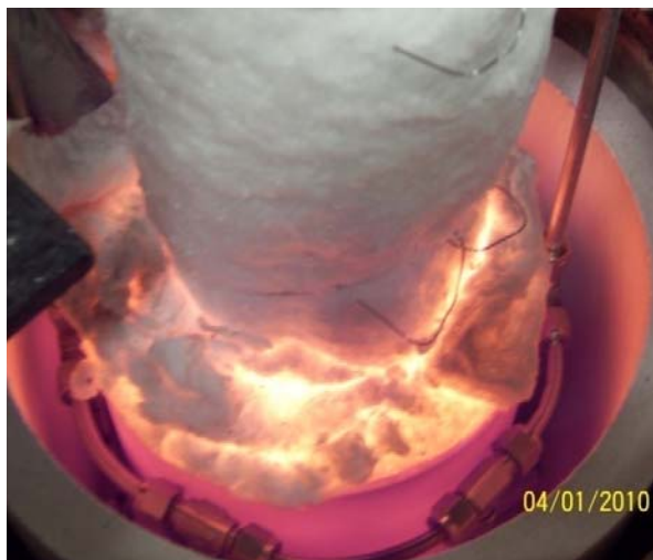
Figure 10. Appearance of the stainless container/graphite crucible/ melter tube assembly in the induction furnace when the temperatures were 1313 °C inside the graphite crucible, 714 °C on the inside of the stainless steel container, and 1080 °C inside the melter tube (measured by a thermocouple immersed in the melt).
