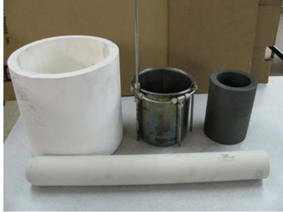
Figure 3. Ceramic safety crucible (left), stainless steel can (middle) and graphite crucible (right) and ceramic melter tube (in front) used in both induction melting experiments. The stainless can, graphite crucible, and ceramic melter tube were placed inside the large ceramic safety crucible.
