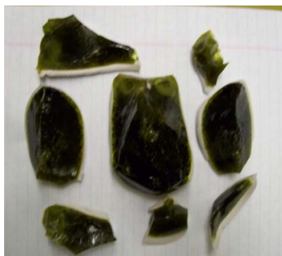
Figure 12. Chunks of the colored BS AN-104 glass that had been melted and let cool.
