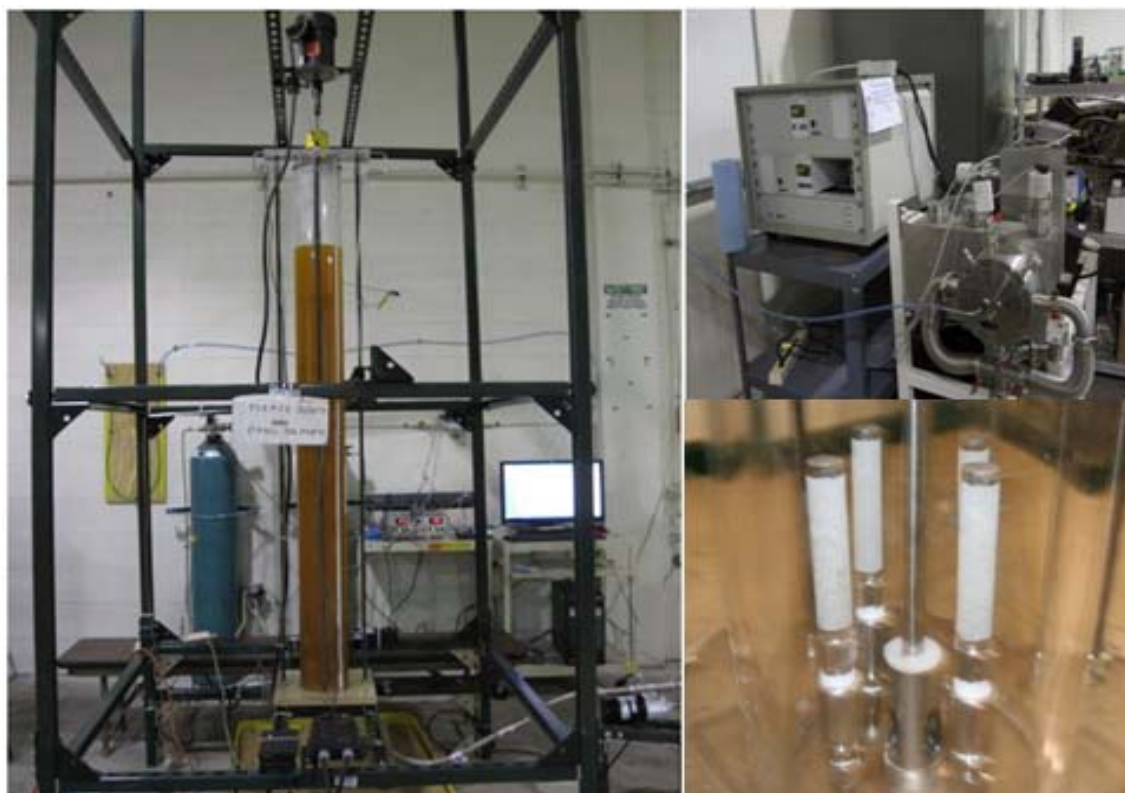
Fig.2. Experimental Set-up (left), mass spectrometer (top right), and spargers (bottom right)
