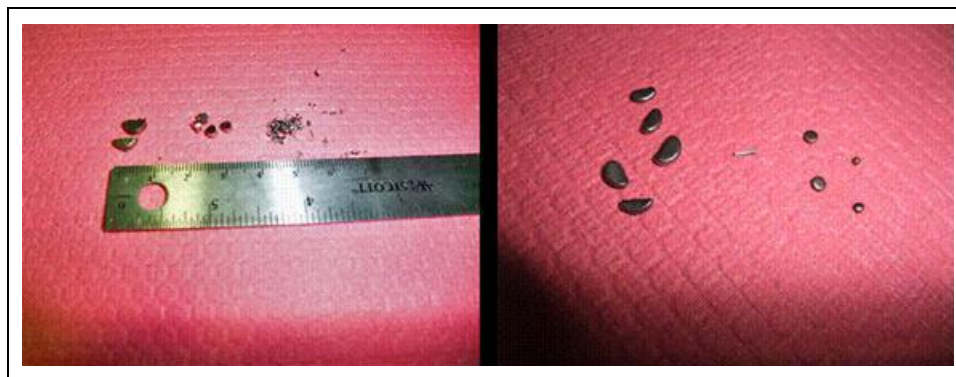
Fig. 4. Starting Coarse, Medium and Fine Densalloy (left). Rounded Densalloy Following Milling (right).
