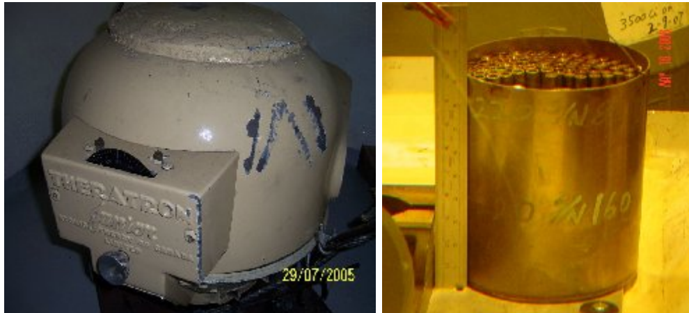
Figure 2: Recovered Co-60 Device and Sources in Hot Cell
