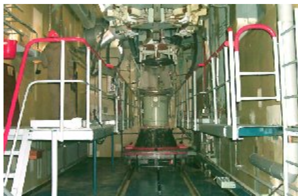
Fig. 2 Feeder and transport system of rotary thin-film evaporator
