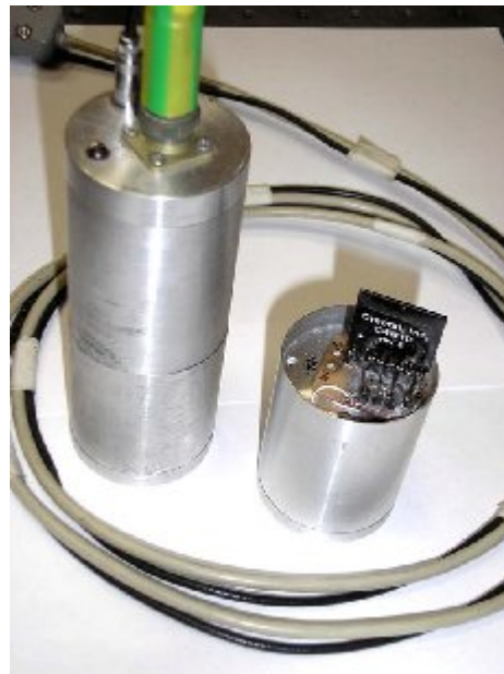
Fig.2 The detectors scintillator CsI(Tl) – PIN photodiode
