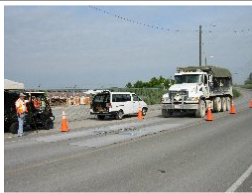
Figure 4. Dump truck approaching portable WIM (testing at ETPP).
