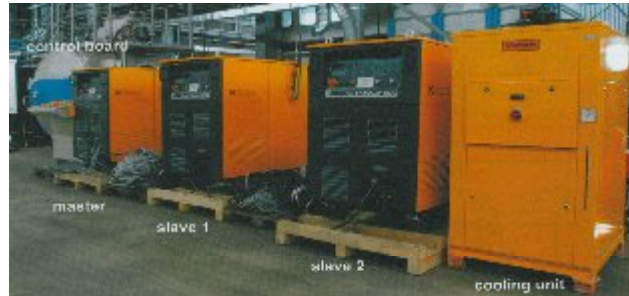
Fig. 2: Plasma power sources with control board, cooling unit and supply lines
