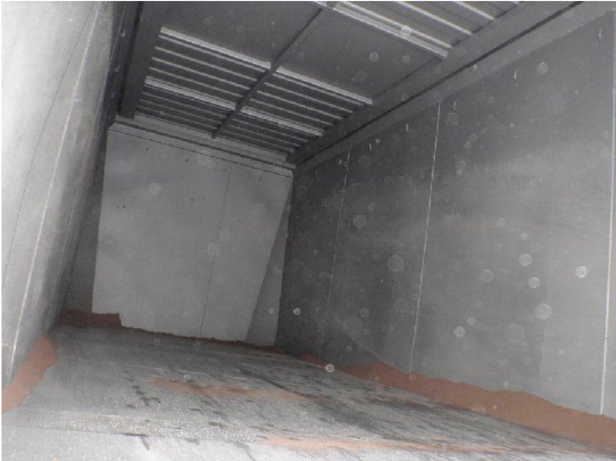
Figure 3. Photograph of container with spray-in liner after unloading.
