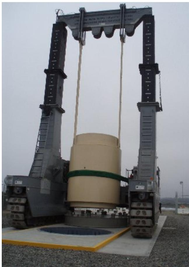
**Figure 18 - VCT Preparing to Lower a HI-STAR HB into the ISFSI Vault**
