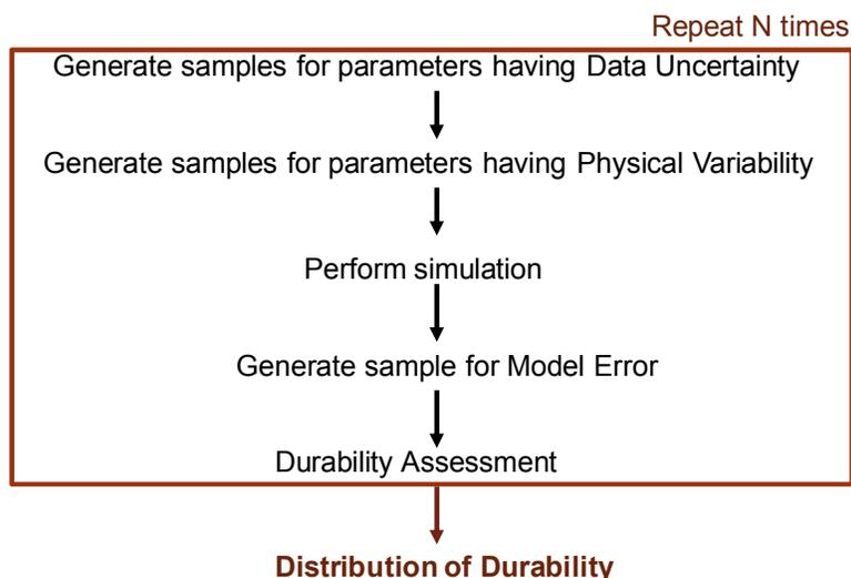
**Figure 2: Probabilistic durability assessment using single loop Monte Carlo simulation.**
