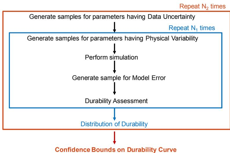
**Figure 1: Probabilistic durability assessment using nested Monte Carlo simulation.**
