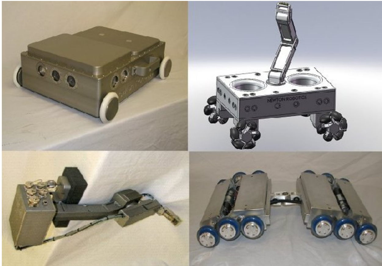
Fig. 4. Examples of robots designed for specific purposes: Clockwise from the upper left: Surveyor data gathering robot; Concrete Removal robot using high pressure water jets; Bridge and Sign inspection robot; Valve Seat inspection robot for hazardous areas
