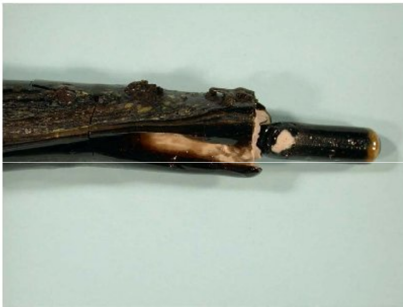
Figure 5. Photograph of a melter suction sample from the end of the test with the original feed blend. The bottom part of the ceramic tube was removed to expose the glass inside. Note patches of yellow phase (originating from the melt surface) and orange-brown material on the far right tip (originating from the melter floor). White material is the ceramic sampling tube.
