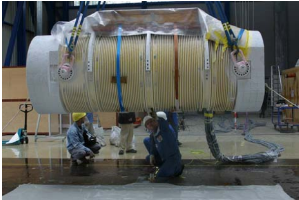
Fig. 1. Preparation of 1m punch test at -40^{\circ}\text{C} (check of test parameters)
