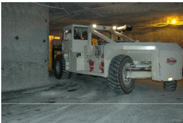
Fig. 1. 41-Ton Forklift going around a corner in the underground repository
