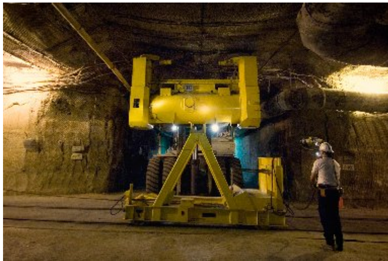
Fig. 5. Facility Cask being lifted from the transfer car near roof
