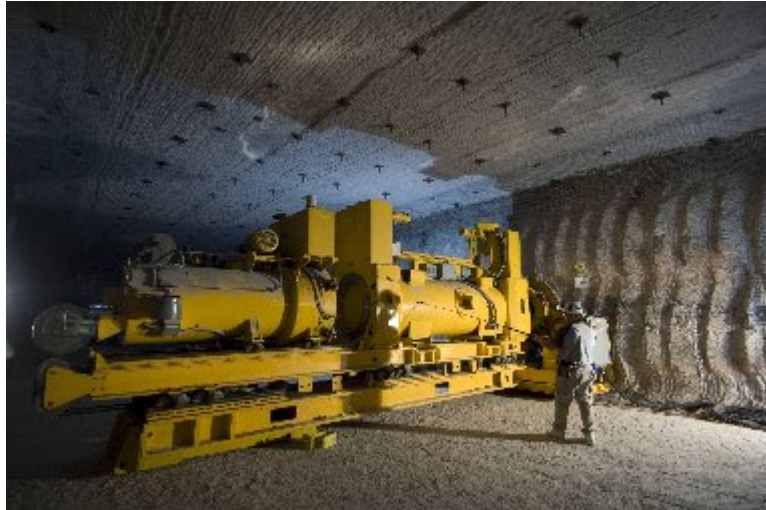
Fig. 4. Facility Cask mounted on the HERE at the disposal borehole
