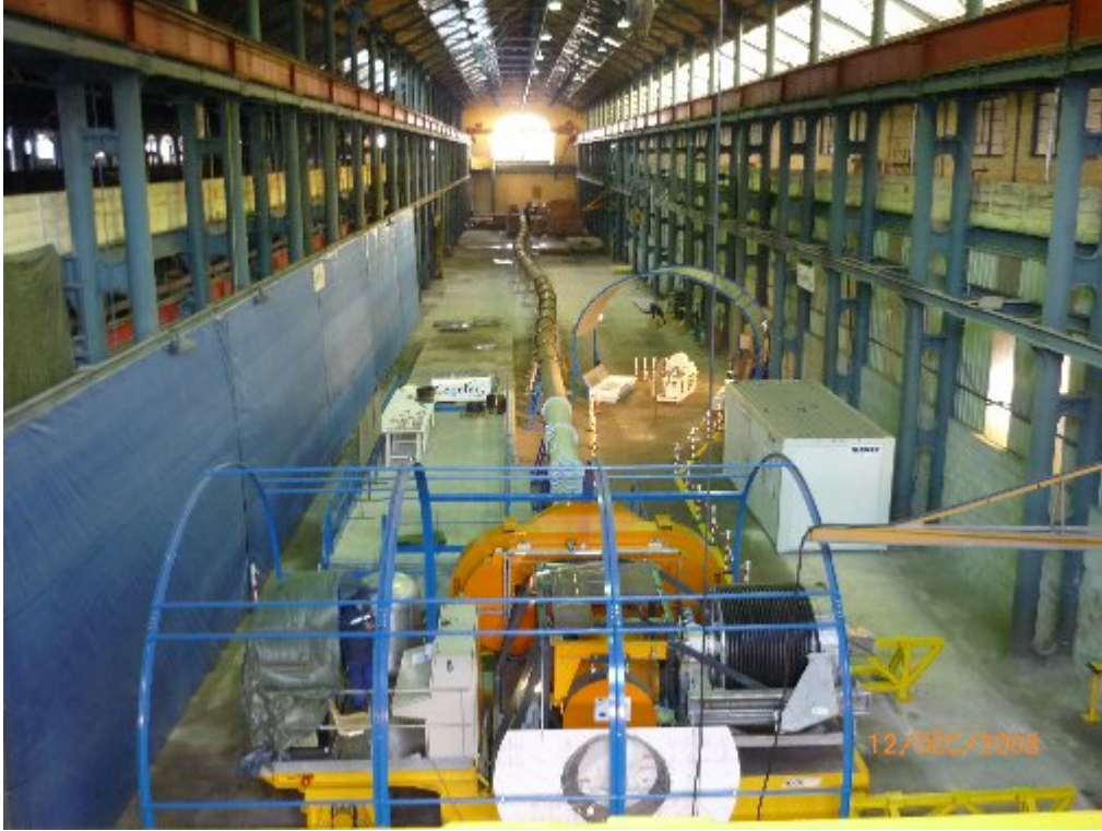
Fig. 6. Pushing Robot Demonstrator tested with a mock-up liner in an S type configuration
