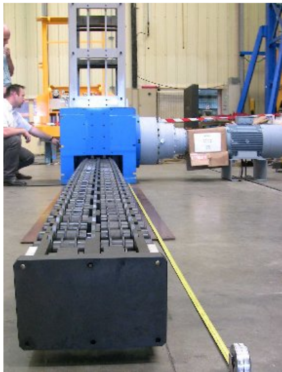
Fig. 7. The Push Pull Chain (fully extended) and its box at rear
